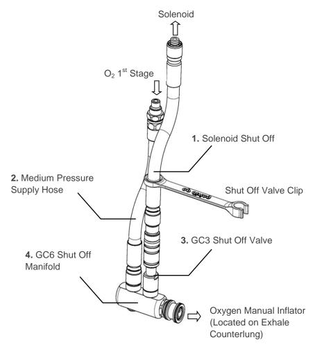
IMPORTANT: You must ensure you connect the hose between the Solenoid and the GC3 Flowstop (Shut Off Valve) the correct way round. The hose ends are shown below.
