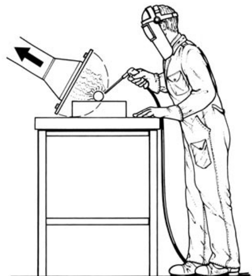
LEV used to help draw welding fume from the breathing zone of a welder
