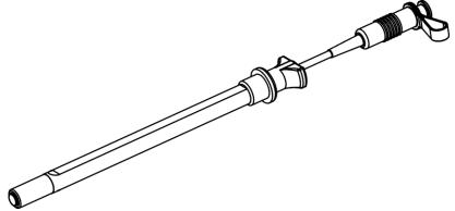
The central rod of the scrubber is replaced by the 'Temp-Stik'; a similar rod with internal temperature sensors, connected by a cable. This is a plug and play device. Inside the scrubber lid is a spare connector: connecting this to the corresponding connector on the temperature stick activates the software so the scrubber monitor is shown in the top centre of the wrist-mounted display.
