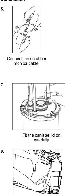
When re-inserting the scrubber assembly ensure the Velcro band passes between the scrubber wall and the down pipe
