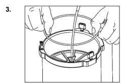
Ensure this O ring is undamaged, clean, lightly lubricated and properly located. Also check for any dirt or damage on the top of the cartridge and place the O ring on top.
