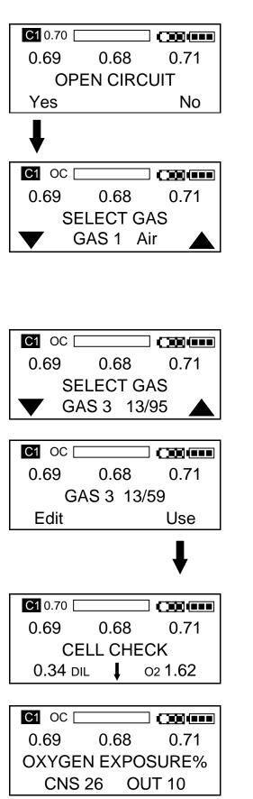
In all version except Dive Timer the first screen displayed in the underwater menu is an option to switch to Open Circuit Decompression.
