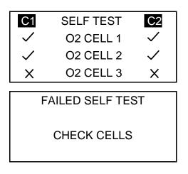
If a cell is not seen by both controllers then the electronics will not go into Dive mode and the connection or solenoid must be fixed prior to use.
