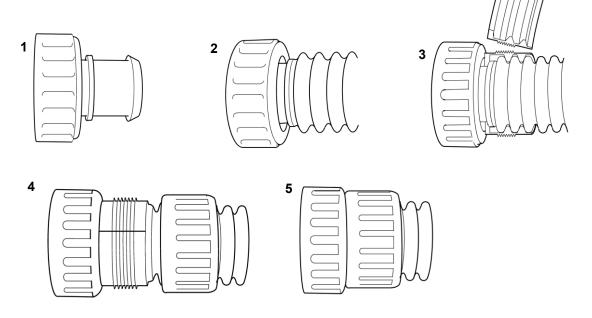
1 & 2: Push the coupling into the hose until the hose is against the first lip of the fitting.
