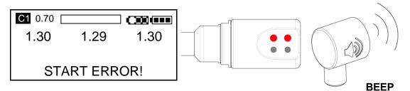
If the electronics are switched on and the pre-dive sequence is not completed and the diver enters the water, once below 1.2m(4ft) the dive Start Error will be displayed.
