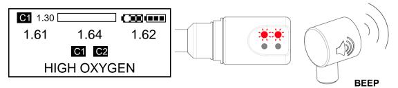
The HIGH OXYGEN warning is set at 1.6 bar. One or both red lights flash **quickly**, the buzzer sounds and "HIGH OXYGEN" is displayed alternating with  $ppO_2$ , depth and dive time information. The warnings will continue until the  $ppO_2$  drops below 1.6 bar.
