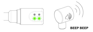
When the setpoint changes from high to low the HUD will give a double Green flash and the buzzer will give a double beep audible alarm.
