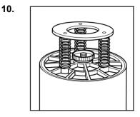
Do not over-tighten the retaining nut
