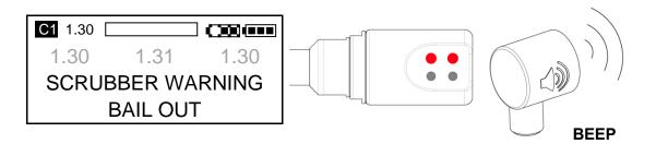
**NOTE:** The Scrubber warning system does not measure CO<sub>2</sub>, it monitors scrubber activity by measuring the temperature throughout the Sofnolime bed.
