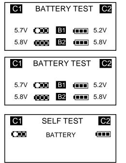
The solenoid "load" is placed on each battery compartment in turn and the battery voltage will be seen to drop. Each battery compartments voltage is measured by both oxygen controllers, C1 and C2. This test is designed to help eliminate weak batteries before you enter the water.
