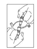
Carefully disconnect scrubber monitor cable and only fit protective covers when dry.
