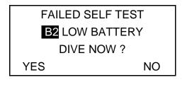
This warning screen shows battery B2 as low or missing. If YES is selected to DIVE NOW the Battery Test Screen will appear as before. A further warning screen will appear after the solenoid "load" test has been conducted.
