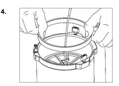
Ensure the spacer ring is clean and undamaged and place carefully onto the O ring. Again push down and ensure the cartridge is free to move up and down and check for the spring loading effect of the pressure spider. If the spacer ring is marked on one side, turn it over to ensure the good side sits on the O ring. Should both sides of the spacer be marked, replace the spacer with a new one before diving.
