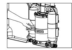
Pull apart the Velcro strap surrounding the canister releasing the Canister from the casing
