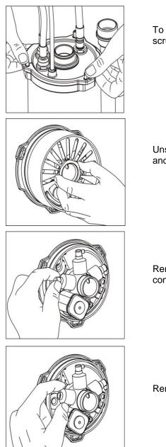
To replace the oxygen cells it is necessary to remove the scrubber from the rebreather.
