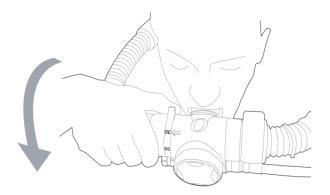
The two modes are selected by rotating the lever forwards or backwards, which in turn rotates the internal components within the main body. The Rebreather mode is activated by rotating the lever to the backward position where the lever is in line with the mouthpiece. The Open circuit mode is activated when the lever is rotated forward to the 'up' position.
