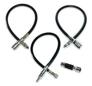
The heart of the gas connection system (GCS) consists of 2 quick release hose fittings, one male and one female. The hose with the male fitting connects to the **ADV** or 2nd stage and the female connects to the intermediate (low) pressure port of your 1st stage.
