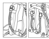
Repeat the process, thoroughly flushing the counterlungs with fresh water
