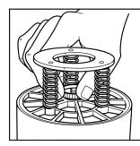
Fasten the retaining nut
