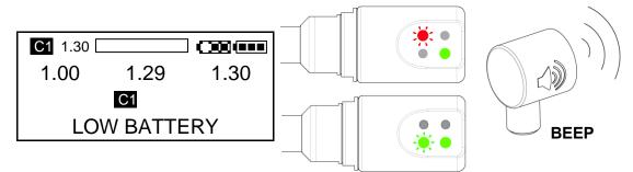
A low battery warning is indicated by alternating red/green/red/green etc flashing lights in C1 or C2 or both if both have low battery levels.
