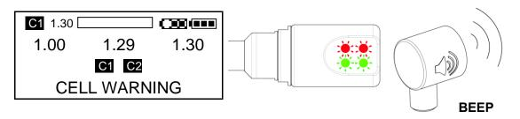
A CELL WARNING occurs if one cell deviates from the average of the closest two by more than 0.2 bar.
