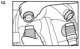
Re-fasten the hoses. Nip them up hand tight. Excessive force does not improve the sealing effect so DO NOT over-tighten.
