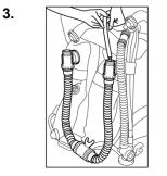
With the mouthpiece closed, use a clean hose to fill both counterlungs with warm, fresh water
