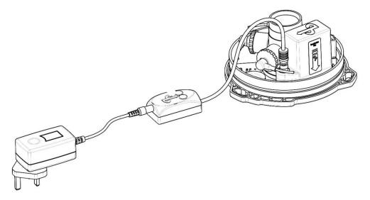
6. The dual charger will light up showing the charge status of each battery within the battery pack.
