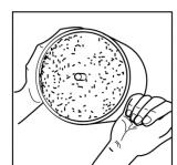
Fill to within 6mm of the top and tap gently on the sides to level the granules
