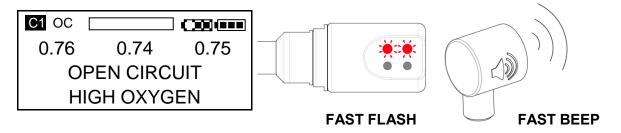
For instance, if you choose an open circuit gas with a  $ppO_2$  greater than 1.6 bar then OPEN CIRCUIT HIGH OXYGEN will be displayed on the handset and HUDs. Similarly, if the gas selected is hypoxic at the current depth (less than 0.2 bar) the OPEN CIRCUIT LOW OXYGEN will be displayed on the handset and HUD.
