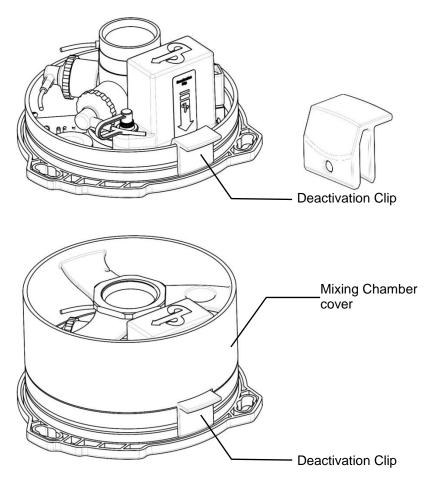
This clip allows the diver to isolate the power supply when flying with the rebreather lid and also avoid the worry of the auto activation turning the unit on unnecessarily when in a damp environment.
