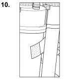
Re-fasten the hoses. Nip them up hand tight. Excessive force does not improve the sealing effect so DO NOT over-tighten.
