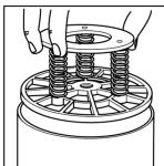
Fit the spring loaded pressure spider
