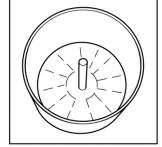
The filter scrim must be located properly in the bottom with no gaps around the edges or the centre column. Its purpose is to retain the Sofnolime granules and keep water out
