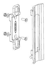
Ideal for attaching cylinders securely and conveniently to the side of the case. It features a strong and easy to operate quick release/attach mechanism. The case-plate is bolted through pre-drilled holes in the case. The cylinder plate, incorporating the quick release/attach mechanism attaches to the cylinder with rubber sleeved "jubilee" clamps (not shown). The case-plate is compatible with the range of Metalsub diving lamps and accessories.
