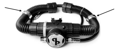
The hose weights should be moved to ensure the mouthpiece sits horizontally, has neutral buoyancy and sits comfortably in your mouth. e.g. If the mouthpiece is digging into your top lip, either the hoses are twisted or the mouthpiece is too buoyant in which case moving the hose weights towards the mouthpiece ensures better comfort. Conversely, if the mouthpiece is too heavy, move them outwards.
