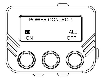
Here the option is given to either switch off completely by selecting ALL or switch on C1.
