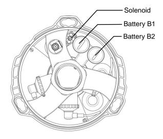
The battery life varies due to the frequency of use of the backlight and the brightness setting. To ensure that the reserve power is as good at it can be and you get the best use from the batteries always discard the batteries in B1 compartment (nearest the solenoid) when the low battery level is reached, replacing them with the two batteries from B2 and inserting new batteries into the B2 slot..
