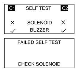
If the solenoid is not seen by both controllers then the electronics will not go into Dive mode and the connection or cell must be fixed prior to use.
