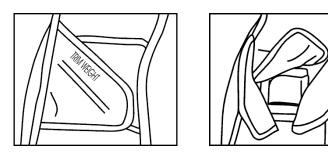
At the waist, mounted on the harness are two large weight pockets with internal removable weight pouches. To prevent un-intentional release, each weight pouch is attached with a 25mm side release buckle making it a 2-stage process to ditch the lead pouch. One pouch has a male fitting and one a female so the two pouches can be clipped together which makes them easy to carry. The weight pouches are loaded from the top through a Velcro flap and shaped with stiffeners to make loading easy.
