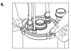
Remove the lid by pulling upwards
