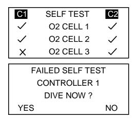
If a cell is missing from one controller, that controller will not be active as a Master.
