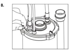
Lift and turn each catch to lock the lid in position
