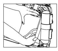
The scrubber locates on the back frame and is held in place by the Velcro band. The inlet pipe MUST sit underneath the cylinder against the back-frame.
