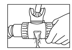
Spray the mouthpiece with disinfectant and thoroughly flush through. Do this with the mouthpiece open and closed to wash the water drain
