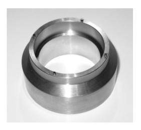
This tool is used for removing and placing back of the locking ring (16) from the T-piece body (5). Using this tool avoids damaging the locking ring, which is not easy to remove using standard pliers due to the small size of the slots and the size of the locking ring.
