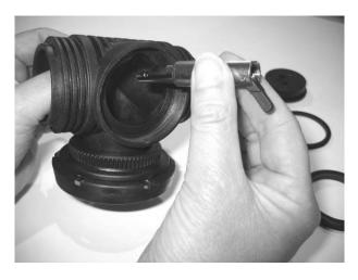
The BS014 O-ring (4) on the outside of the banjo seals on the outer face of the ADV. Make sure you extract the ADV body carefully, without levering.
