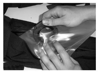
Using RBTOOL 6 to grip the Top (19) and your hand to grip the Retainer Base (23) through the material, unscrew the Top (19).
