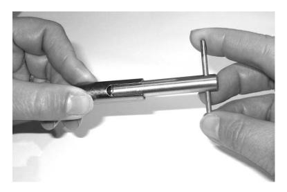
Use the demand valve slotted tool (RB TOOL 7) to screw the tilt boss back into the ADV body (6). Screw clockwise.
