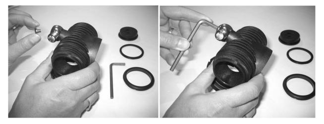
Screw clockwise. Use 5 mm Allen key to tighten until locked against ADV body.
