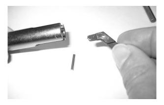
The pin holds its position in the lever solely by friction; no locking rings etc. are used. Make sure you do not damage the plastic lever if you use a small tool to push out the lever pin. Use a pair of pliers to pull the pin out once you can get hold of it.
