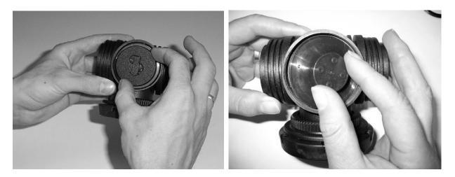
Treat the diaphragm with care. Inspect it carefully for wear and tear. Consider that damage to the diaphragm can lead to a flooded loop of your rebreather! When in doubt, replace.
