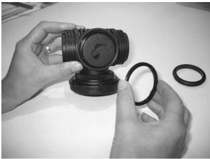
Unscrew counter-clockwise, using special tool RB TOOL 8 or a correct fitting pair of pliers with thin tips. Make sure that the 4 pins from the special tool are properly locked into the 4 small holes in the locking ring to avoid damaging the ring.
