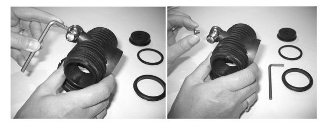
Unscrew counter-clockwise. Use a 5 mm Allen key.
