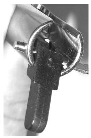
The pin holds its position in the lever solely by friction; no locking rings etc. are used. Try to push the pin in without using tools to avoid damaging it. If you need to use a small tool, make sure you do not damage the plastic lever or the holes in the ADV body.
