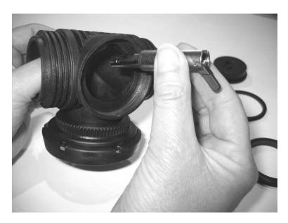
The BS014 O-ring (4) on the outside of the banjo seals on the outer face of the ADV. Make sure you push it through carefully, without levering.
