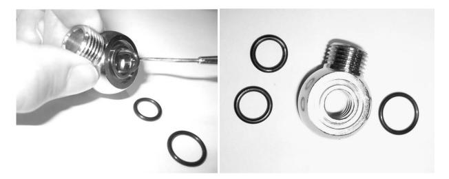
**WARNING:** It is almost impossible to remove these O-rings without damaging them – especially the smaller ones on the inside. Therefore <u>NEVER</u> re-use the old rings; always use new ones!. DO NOT use the Banjo body to lever the O-rings out, this may damage the sealing face.
