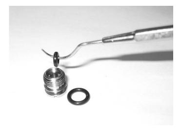
This small O-ring has a very special role. It acts as the valve seat for the tilt-axle which acts as an upstream valve. Together with the tilt-axle they act as the core valve assembly of the ADV. Damage to this O-ring will lead to a leaking ADV. Therefore <u>ALWAYS</u> replace it when servicing the ADV.
