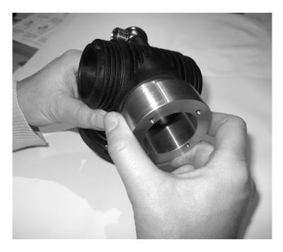
Screw clockwise, using special tool RB TOOL 8 or a correct fitting pair of pliers with fitting thin tips. Make sure that the 4 pins from the special tool are properly locked into the 4 small holes in the locking ring to avoid damaging the ring.
