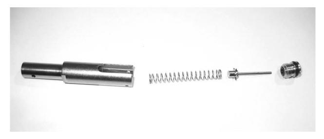
After removal check again if the tilt axle hasn't got bent by the removal process.
