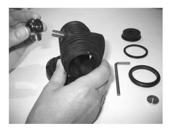
Make sure the BS014 O-ring on the outside of the banjo is facing the T-piece body.
