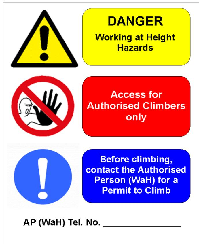
3. All signs are to be clearly displayed on or in the vicinity of each RHP and to be easily visible on the approach to the fixed access.
